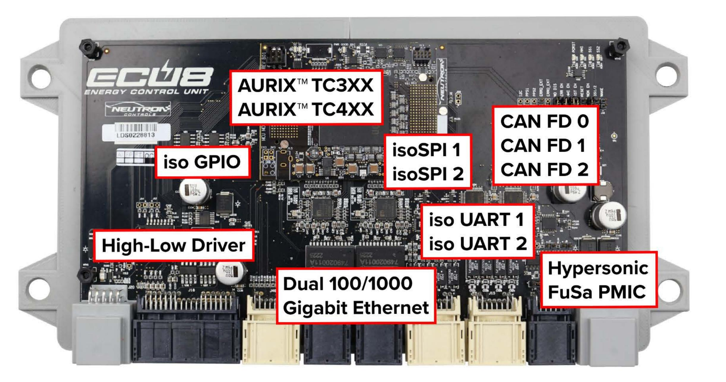
ECU8™ is an AURIX™ based ECU Prototype platform that allows for rapid software development. This ECU design can be modified and customised to meet YOUR production requirements.
