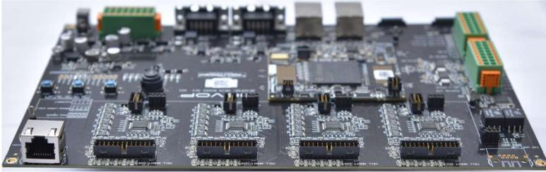
BEVOP™ provides the hardware and software components needed to accelerate the development of a Battery Management System (BMS) for a wide variety of applications including automotive and others with different levels of safety requirements.
